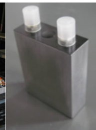
Coda 14.5Ah Li-ion Battery Cell
